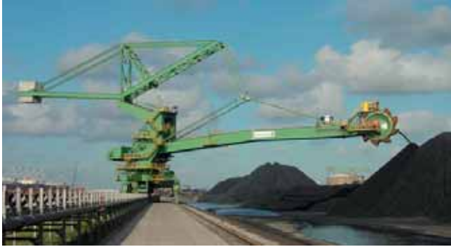
Picture 1.3 : A ThyssenKrupp's high capacity bucket wheel machine working at EMO Terminal Holland, similar to the project
