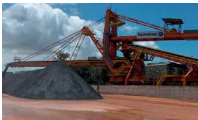
Pictures 1.1 + 1.2: Similar blending yard machines working in an iron ore concentrate plant in Brazil
