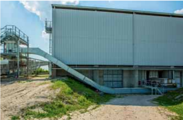
The chain belt conveyor lifts the material to the height of the Pipe Conveyor. (©BEUMER Group GmbH & Co. KG)
