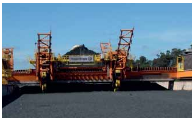
Pictures 1.1 + 1.2: Similar blending yard machines working in an iron ore concentrate plant in Brazil
