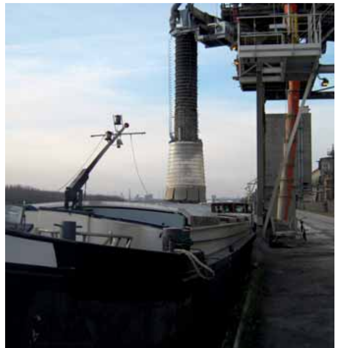
Fig. 4. Combined loading system with pneumatically operated shutter cone for loading of cement on open ships or tank ships.
