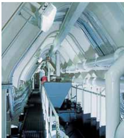
The IBAU HAMBURG Tunnel concept: Midship tunnel with the IBAU Pump and aeration panels.
