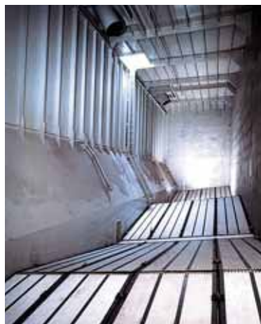
The IBAU HAMBURG Tunnel concept: Midship tunnel with the IBAU Pump and aeration panels.
