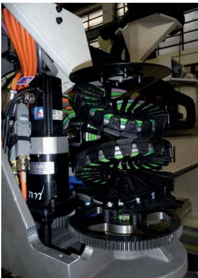
This twisterband can conduct a 1,440° rotation. This application in the wood working sector won the bronze vector award in 2012. (Source: igus GmbH)
