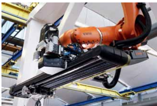
Winner of the golden vector award 2012: the KUKA Cobra. An additional axis is mounted to the robot arm to load and unload presses. A new, special chain guide design from the igus E6 series is used to make the robot structure as compact as possible. (source: igus GmbH)
