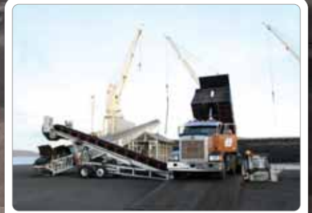
INSTANT PORTABLE TRUCK UNLOADING
