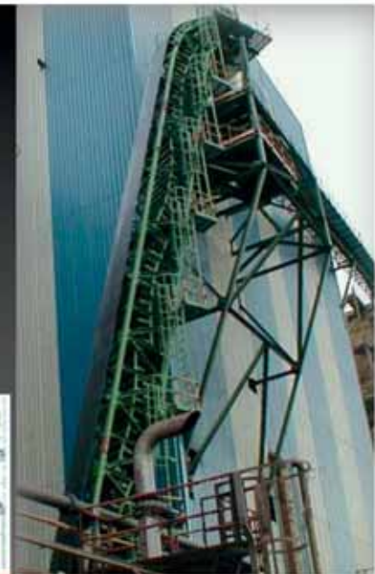
DSI Snake Sandwich High Angle Conveyor elevating coal at a 75° angle for a steel plant in Northern Spain.
