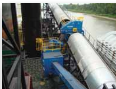
TWO STAGE MECHANICAL SAMPLING
