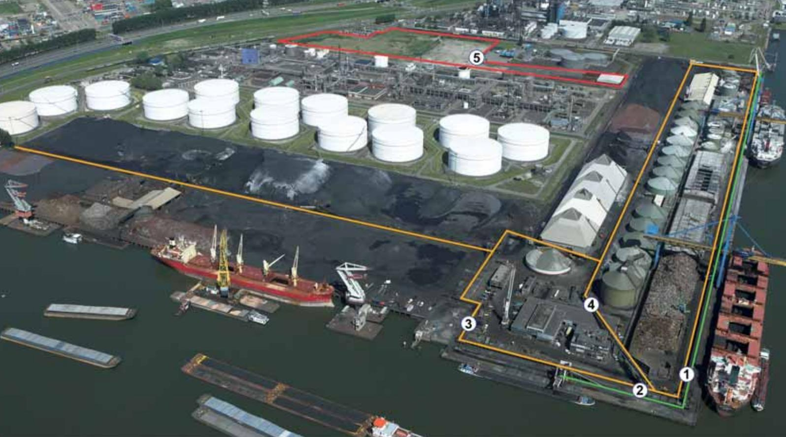
▶ Board-to-board circuit from ocean vessel into coaster/barge (—), magnets 1 and 2, from vessel onto storage circuit (—), magnets 1, 2, 3 and 4. Overbelt magnets 1 and 3 are placed at the transformer points of the conveyor belts.
