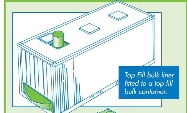
Top Fill bulk liner fitted to a top fill bulk container.
