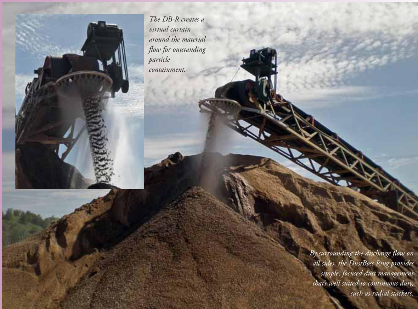
*The DB-R creates a virtual curtain around the material flow for outstanding particle containment.*
