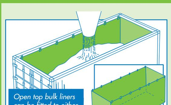
Open top bulk liners can be fitted to either open top containers or bulk containers.
