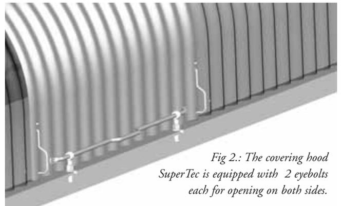
*Fig 2.: The covering hood SuperTec is equipped with 2 eyebolts each for opening on both sides.*
