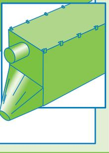
End Fill bulk liner with letterbox discharge sleeve.
