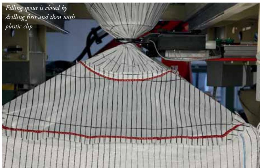
*Filling spout is closed by drilling first and then with plastic clip.*
