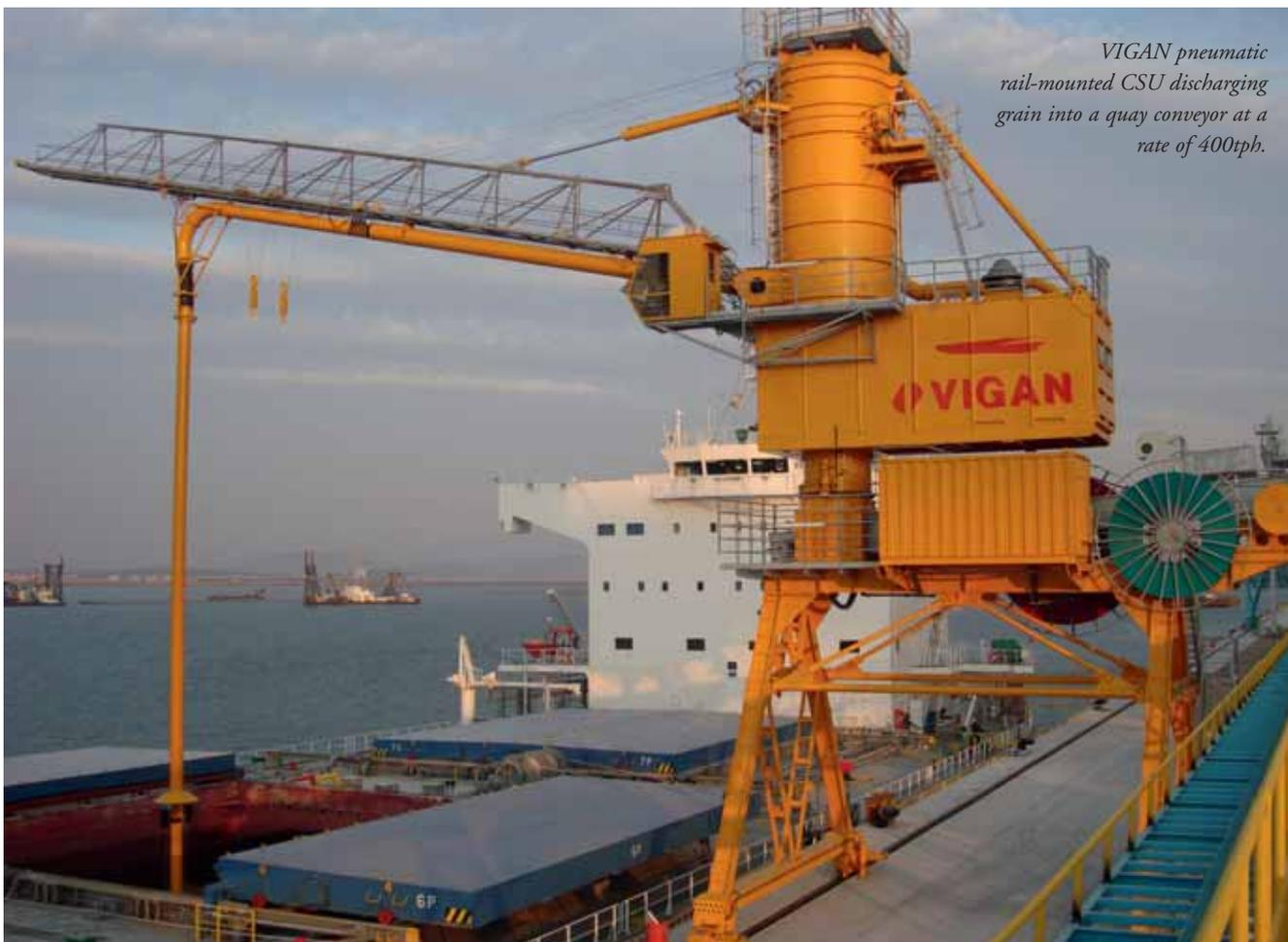
*VIGAN pneumatic rail-mounted CSU discharging grain into a quay conveyor at a rate of 400tph.*
