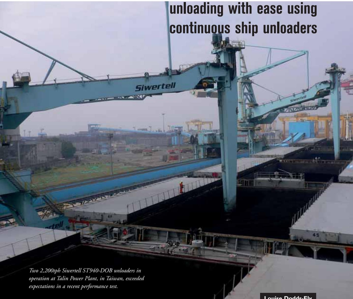
*Two 2,200tph Siwertell ST940-DOB unloaders in operation at Talin Power Plant, in Taiwan, exceeded expectations in a recent performance test.*
