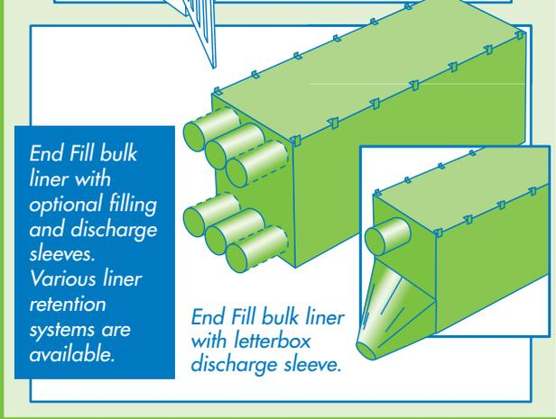
End Fill bulk liner with optional filling and discharge sleeves. Various liner retention systems are available.
