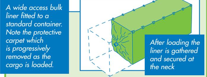
A wide access bulk liner fitted to a standard container. Note the protective carpet which is progressively removed as the cargo is loaded.
