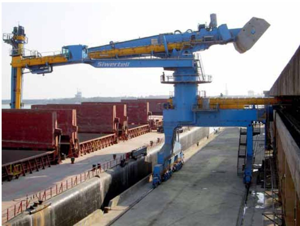
Cargotec has designed a system that reacts immediately upon detection and extinguishes any fire,” Paulsson said. “Fire detectors along the conveying line automatically stop the conveyors and start spraying water from the fire extinguishing system. To manage an explosion, the conveyor’s steel casings are reinforced with extra-thick steel, and explosion-venting valves fitted along the conveyors and dust collectors relieve pressure.”
