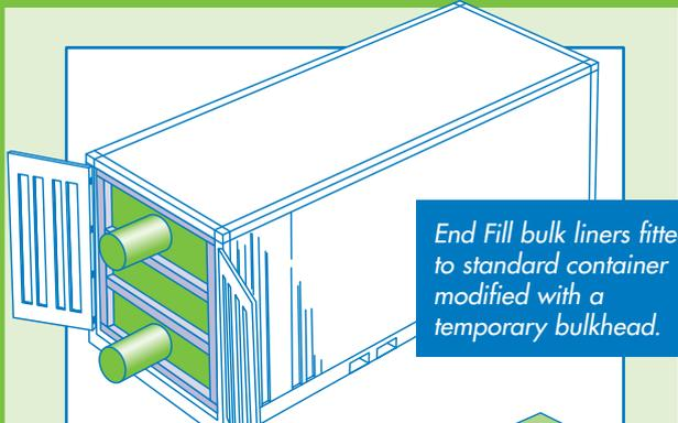
End Fill bulk liners fitted to standard container modified with a temporary bulkhead.
