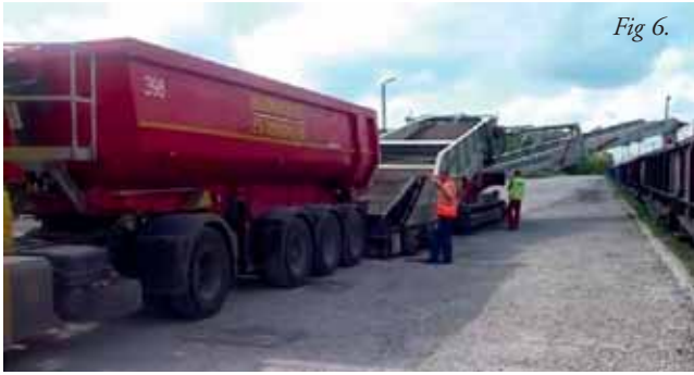
TU 515R mobile radial truck unloader loading rail wagons directly from trucks.
