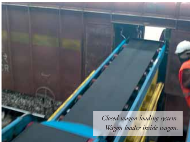
Closed wagon loading system.
