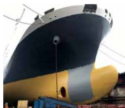
Nippon Paint Marine's self-indicating epoxy coating NOA10M was the coating most frequently applied during the period.
