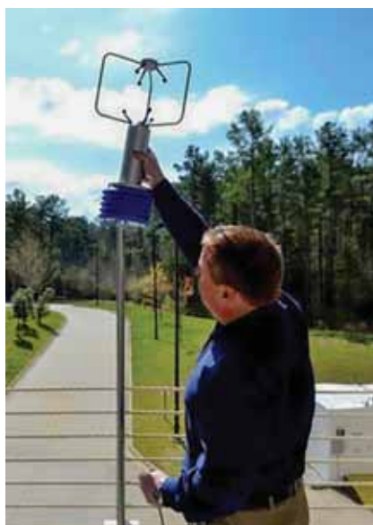
Air quality testing equipment contains sensors that measure microscopic particulates (source – Environmental Protection Agency).
