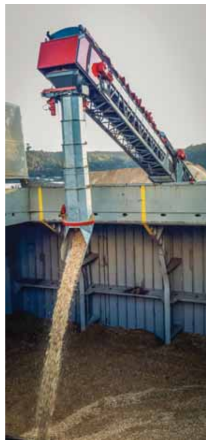
The TB58 Telescopic Shiploader has an extended 58m length conveyor and 8m telescopic discharge chute.
