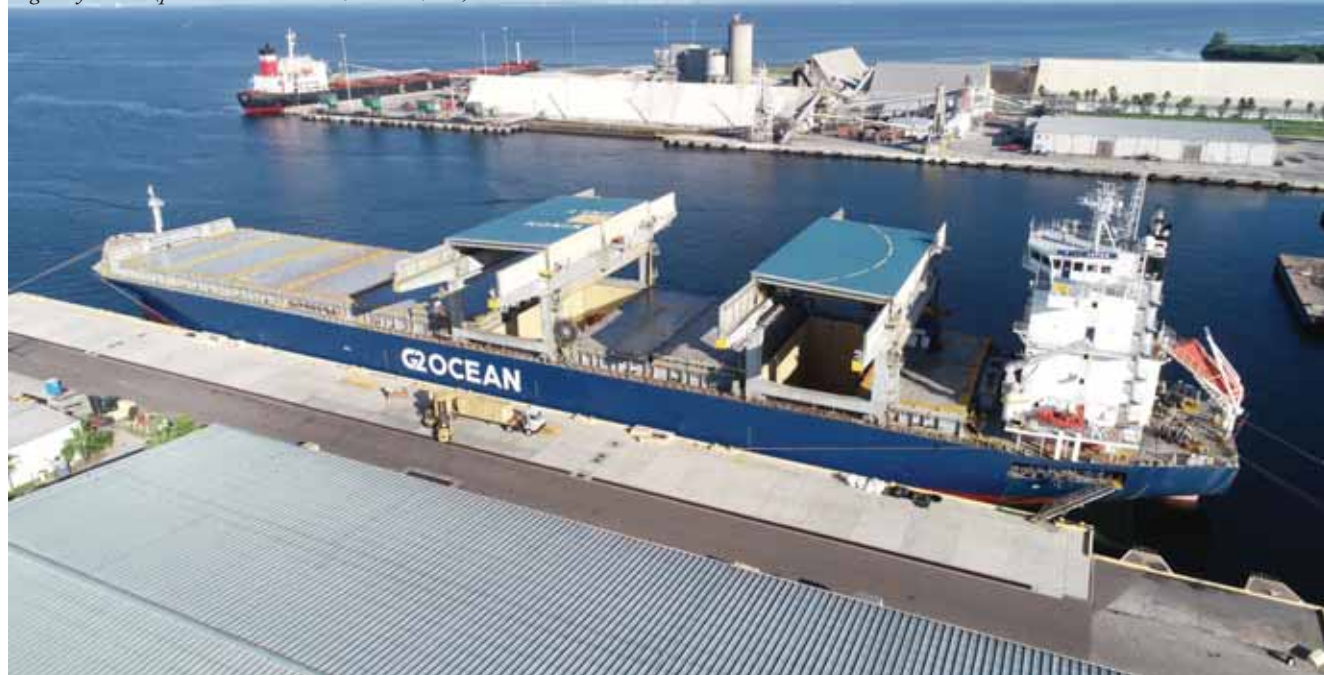
G2 Ocean's gantry crane vessels each have two gantry cranes (photo: Port Matanee, Florida, US).
