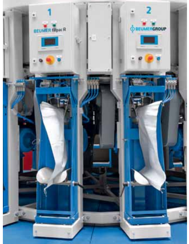
The rotating filling machine BEUMER fillpac R with sophisticated weighing electronics.
