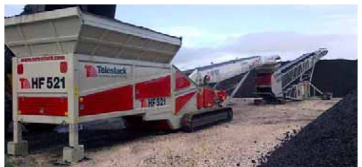
Hopper Feeder & Radial Telescopic reclaiming/ stockpiling coal in stockyard of powerplant
