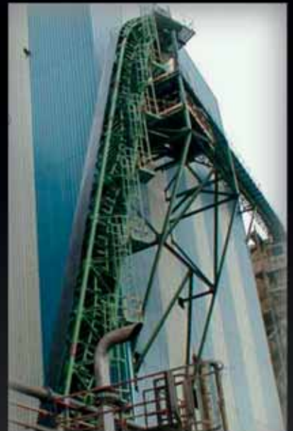
DSI Sandwich Belt High Angle Conveyor elevating coal at a 75° angle for a steel plant in Northern Spain.
