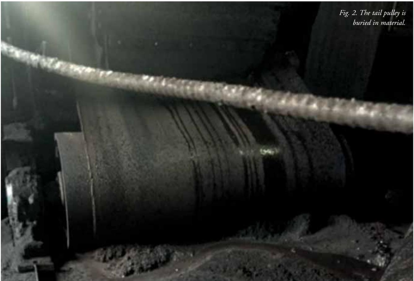
*Fig. 2. The tail pulley is buried in material.*
