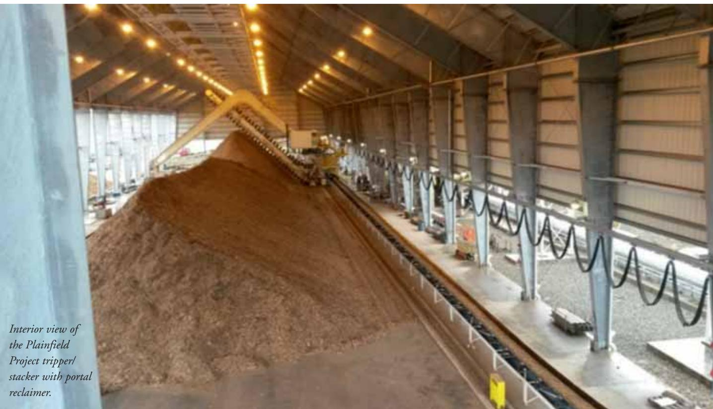
Interior view of the Plainfield Project tripper/stacker with portal reclaimers.
