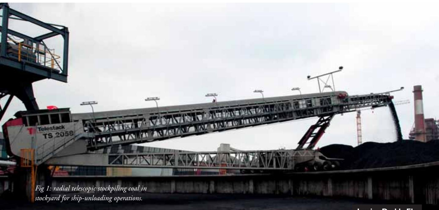
Fig 1: radial telescopic stockpiling coal in stockyard for ship-unloading operations.
