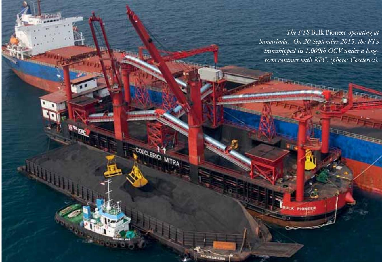
belt measuring each grade flow rate and on the transversal conveyor measuring the total flow. The homogeneous blending of coal is also enhanced by the transfer points of the conveyor system and the revamped system is able to guarantee reliable loading rate from 1,500tph (tonnes per hour) up to 2,000tph. The system is also supported by a sophisticated online sampling device and a metal detector.
