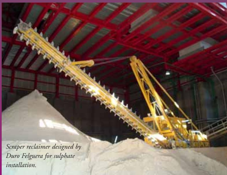
*Scraper reclaimer designed by Duro Felguera for sulphate installation.*
