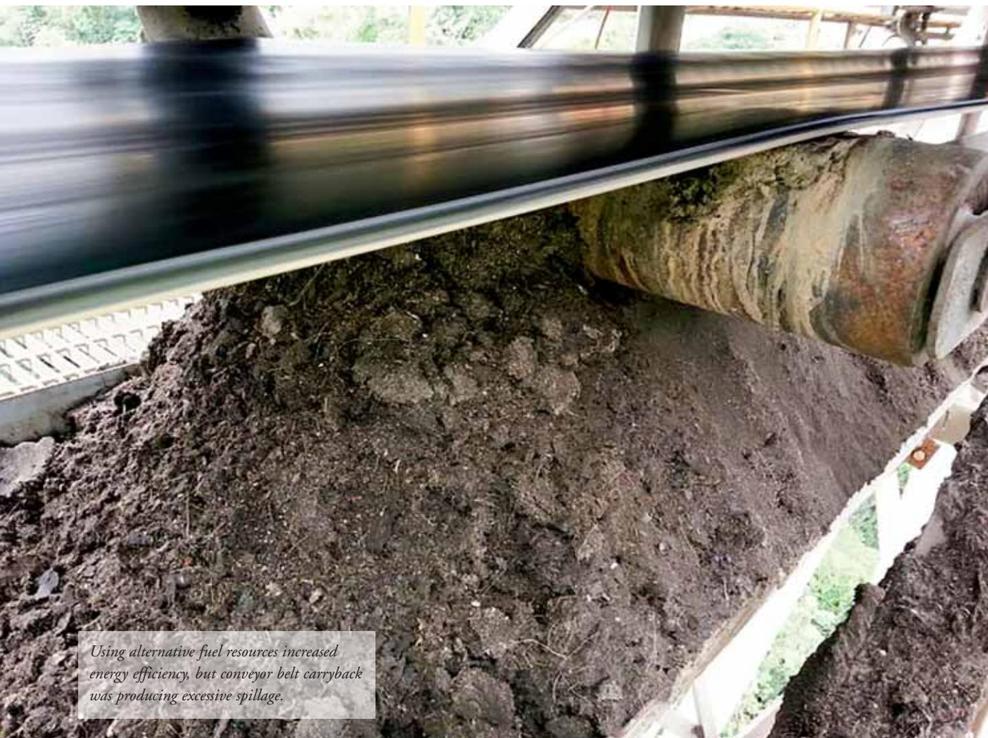
*Using alternative fuel resources increased energy efficiency, but conveyor belt carryback was producing excessive spillage.*
