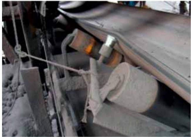
Fig. 3. Ordinary training idler tied off with a rope causing material build up on the support frame work and belt edge damage from friction and pressure.
