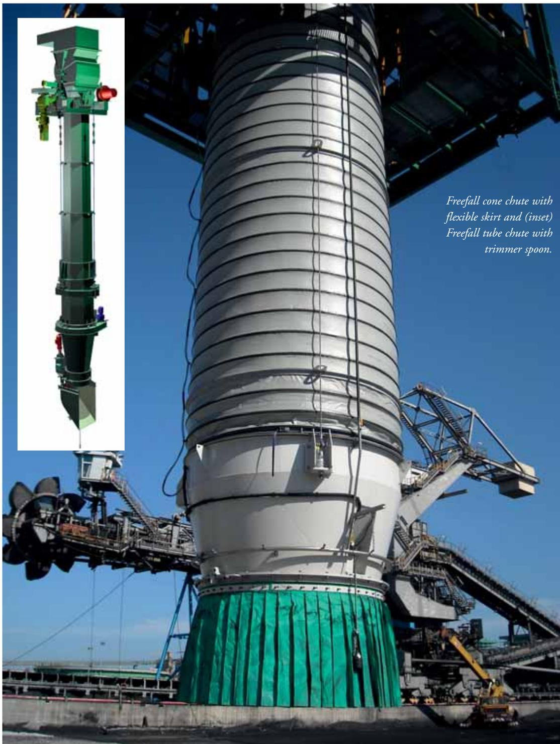
*Freefall cone chute with flexible skirt and (inset) Freefall tube chute with trimmer spoon.*
