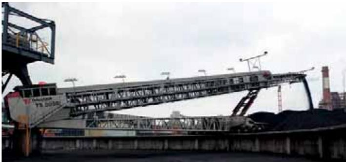
Radial telescopic stockpiling coal @ 2000tph
