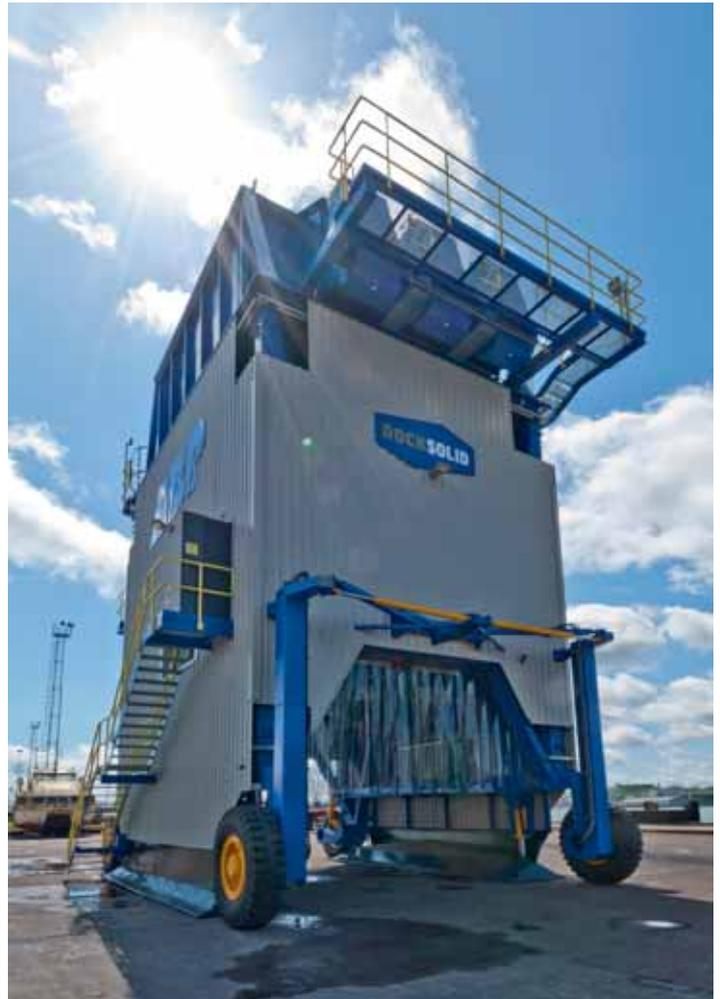
discharge chute, maintaining a negative air pressure and pulling practically all emitted dust particles through a special fabric 'sock' filtration system. A compressed air reverse-jet pulse then periodically cleans the filtration fabric, and returns the collected dry particles to the bulk commodity, for discharge to trucks, rail-wagons or conveyors.
