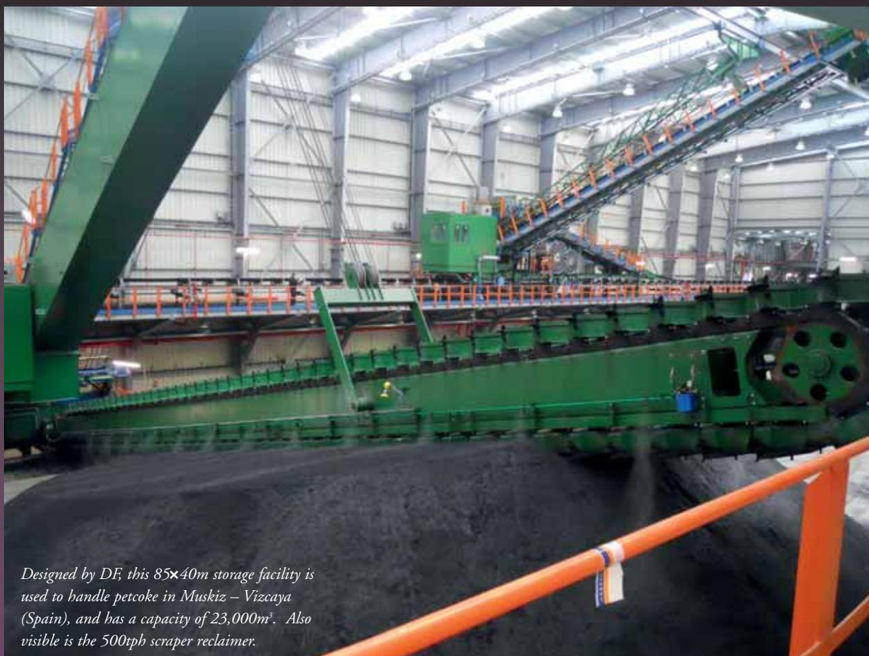
*Designed by DF, this 85x40m storage facility is used to handle petcoke in Muskiz – Vizcaya (Spain), and has a capacity of 23,000m<sup>3</sup>. Also visible is the 500tph scraper reclaimer.*
