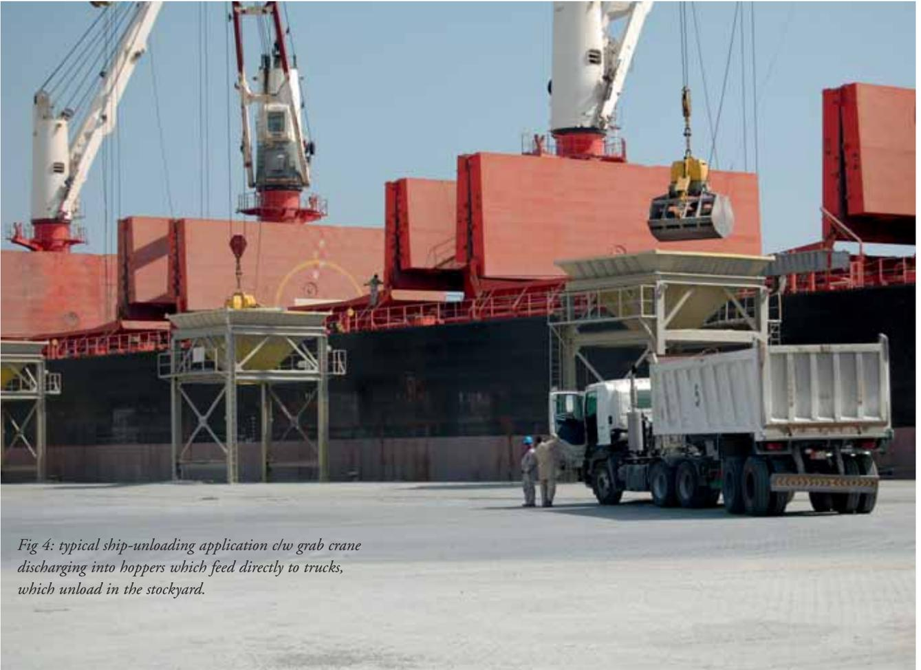
*Fig 4: typical ship-unloading application cw grab crane discharging into hoppers which feed directly to trucks, which unload in the stockyard.*
