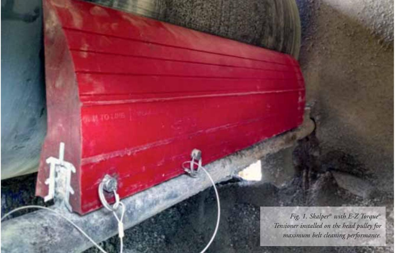
*Fig. 1. Skalper® with E-Z Torque® Tensioner installed on the head pulley for maximum belt cleaning performance.*
