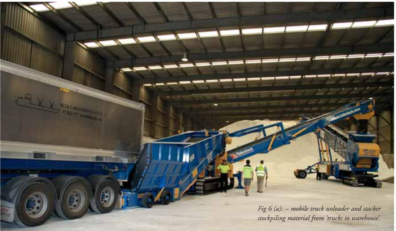
*Fig 6 (a): – mobile truck unloader and stacker stockpiling material from ‘trucks to warehouse’.*
