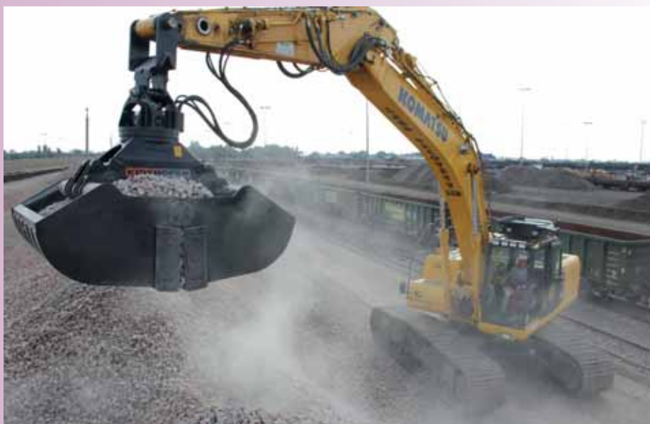
The Kinshofer C40HD Rehandling Clamshell Bucket in heavy duty action at a Network Rail Recycling site in Cambridgeshire.
