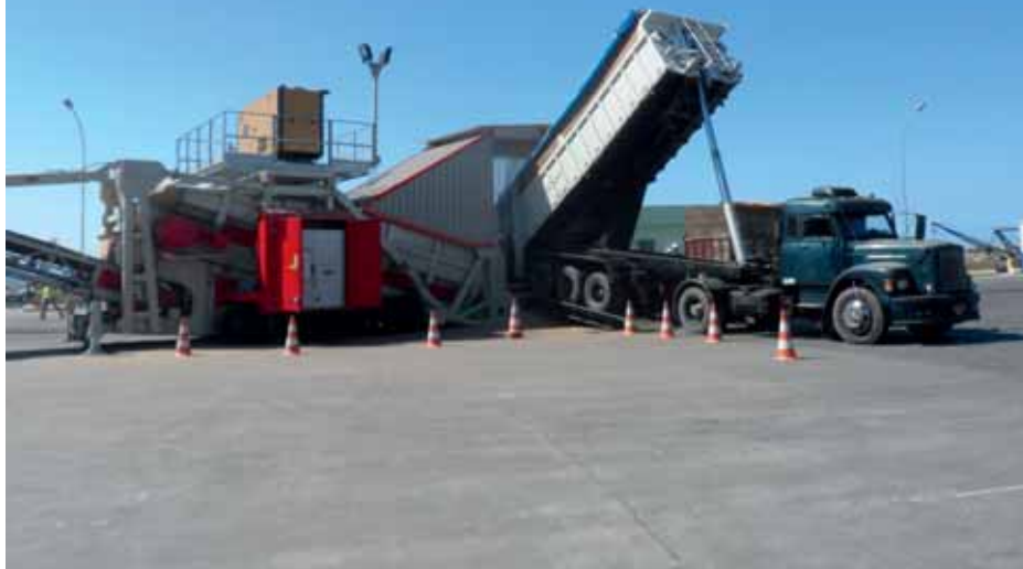
Telestack TU 1016R innovative triple-entry truck feeder points ensure constant flow of material to the Telestack shiploader.
