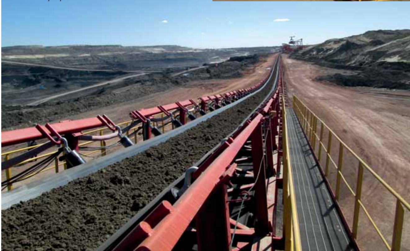
The 7,900m 3 /h Tenova TAKRAF conveyor system at Zhabanaoer open pit mine in China.
