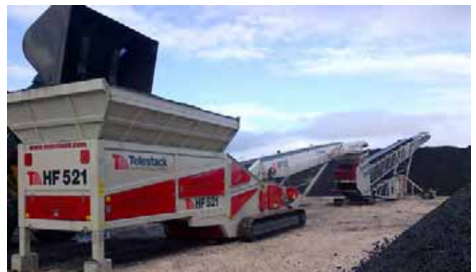
Hopper Feeder & Radial Telescopic reclaiming/ stockpiling coal in stockyard
