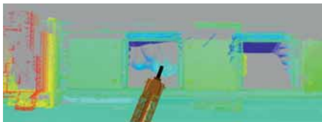
Combination of the iSAM® 3D ship model and a 3D CAD model of a shiploader, displayed as the operator interface, exemplary.
