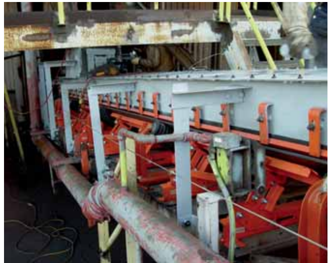
The cradles are designed to be located at transfer points of receiving conveyors, under the hopper and chute box, close to the tail pulley.
