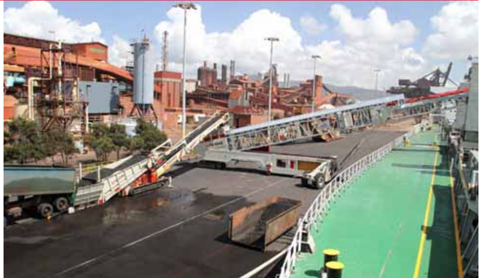
Radial Telescopic Shiploader and Mobile Truck Unloader loading pet coke to handymax vessels
