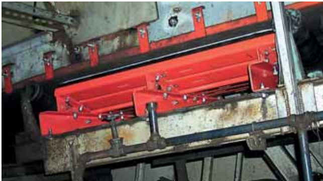
Martin® Impact Cradles feature a bed of steel angles lined by energy-absorbing bars with a top layer of ultra-high molecular weight (UHMW) plastic.
