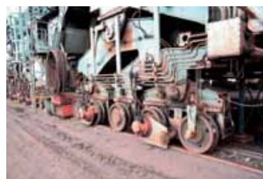
Two of a total of 18 Hägglunds CA motors on the long travel drives of this ship unloader at EECV.
