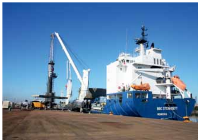
TPP's new Liebherr Pactronic LHM 600 crane is expected to increase its loading rates to 40,000 tonnes per day.
