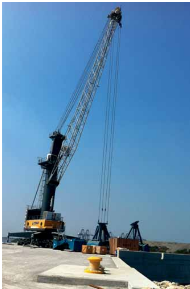
TPP's new Liebherr Pactronic LHM 600 crane is expected to increase its loading rates to 40,000 tonnes per day.
