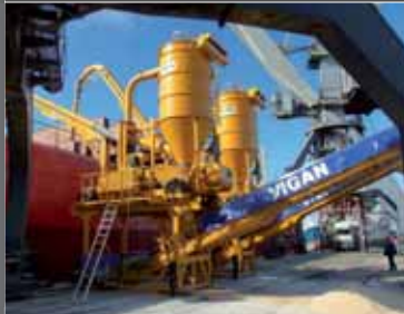
PORTABLE GRAIN PUMPS up to 270 t/h
