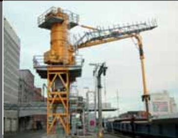
PNEUMATIC UNLOADER up to 600 t/h
