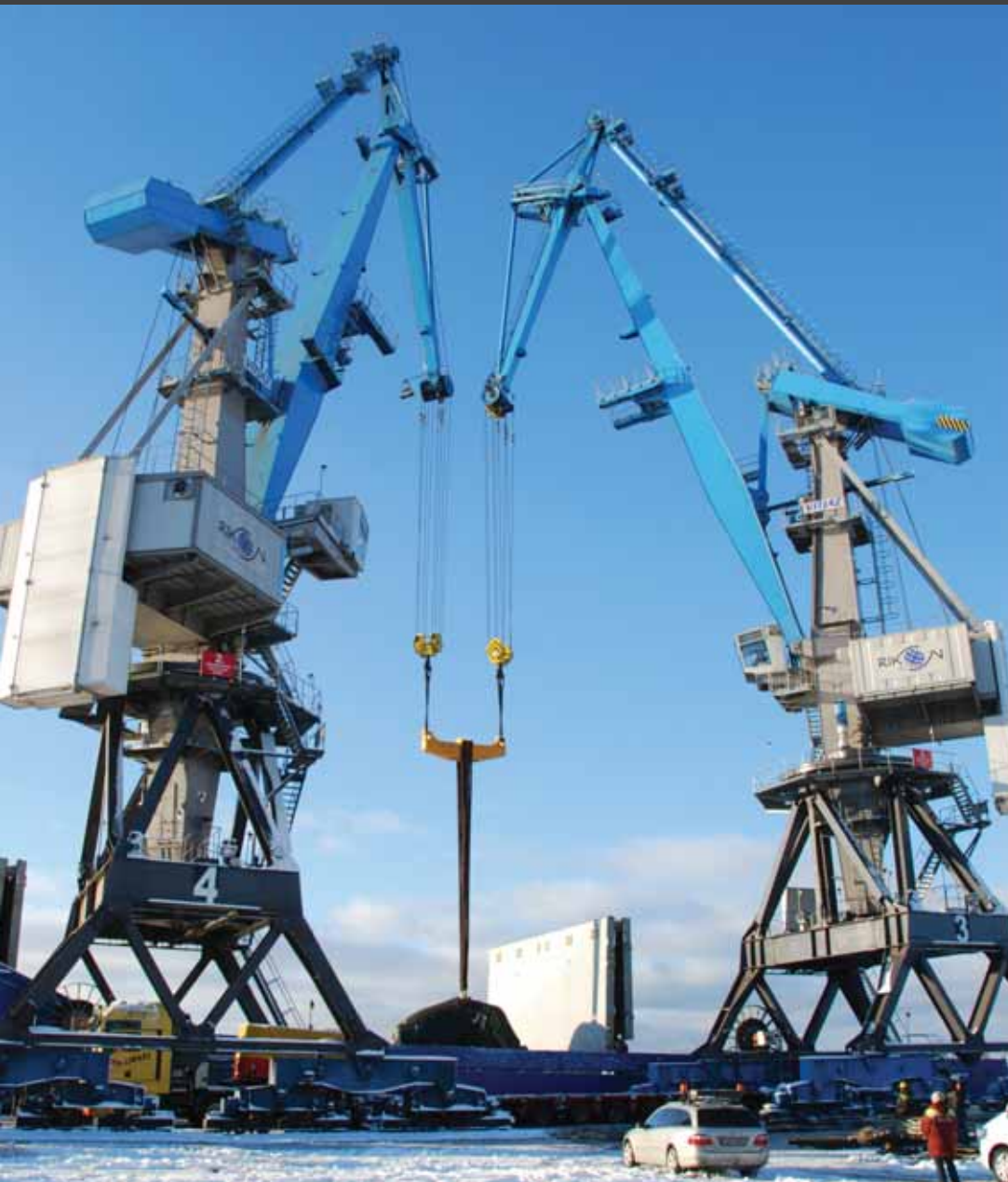
Unloading of 151t turbine in crane tandem mode
