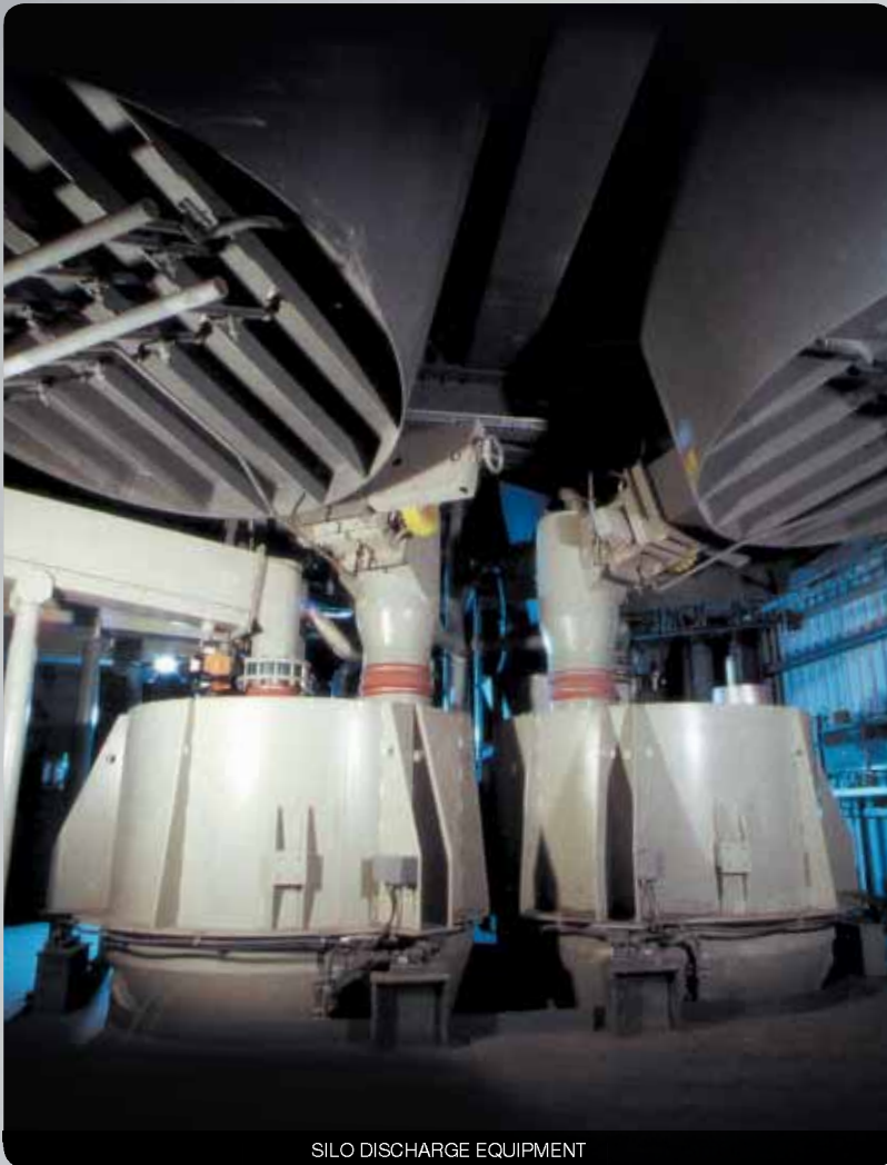
SILO DISCHARGE EQUIPMENT
