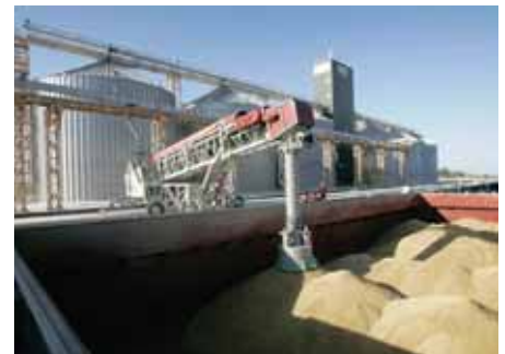
Rail mounted, parallel travel, telescopic conveyor loading grain in Ukraine @ 250tph.
