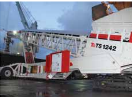
Telescopic shiploader with dust containment & cascade chute, loading PetCoke in Brisbane.
