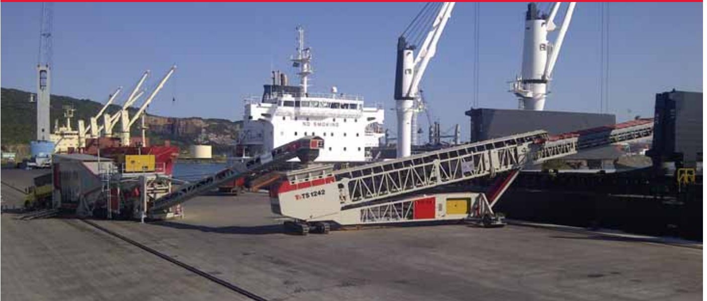
Radial Telescopic Shiploader fed from a triple entry mobile truck unloader in Brazil.
