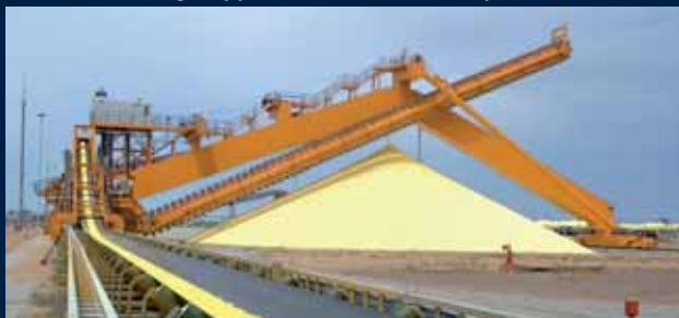
Combined Stacker / Reclaimer, sulphur prills
