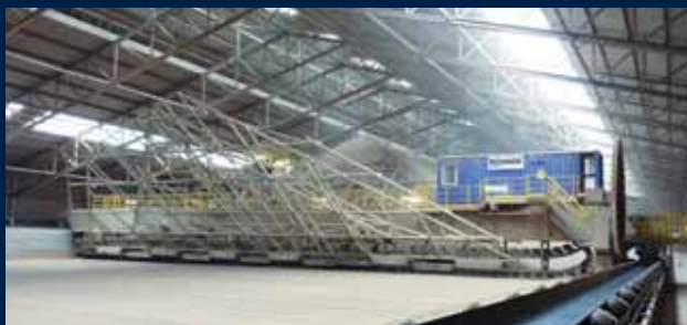
Bridge-type Reclaimer, wood pellets
