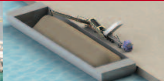
Truck - Truck Unloader - Barge
