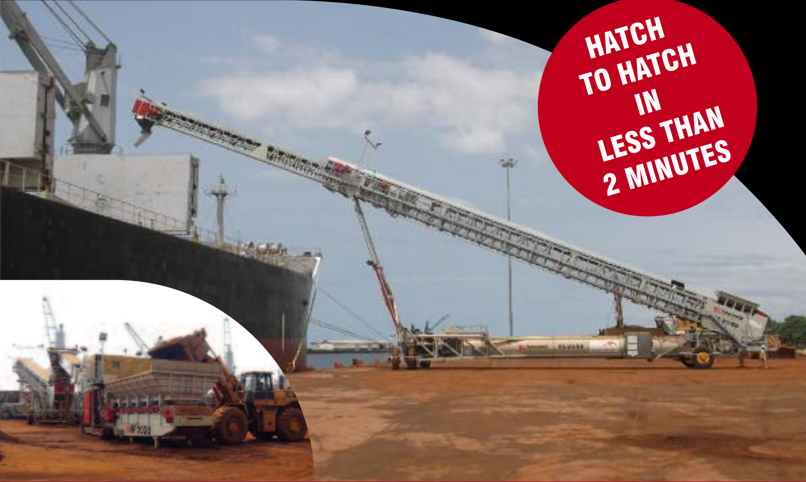
Mobile Hopper directly feeding the Shiploader
