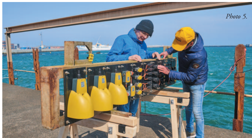
Photo 4: Deep dive and pressurizing: waterproof tests of foot switches in the steute lab (and, below, in situ).
