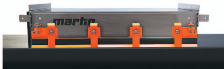
Figure 4: the choice of one- or two-piece Martin® ApronSeal™ Urethane Skirting depends on the available space along the belt edge.
