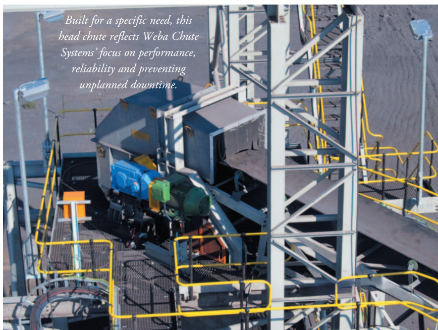
This head chute, which feeds into a bin, is designed to control the speed and direction of material flow, cutting down on wear, spillage and downtime in tough mining conditions.
