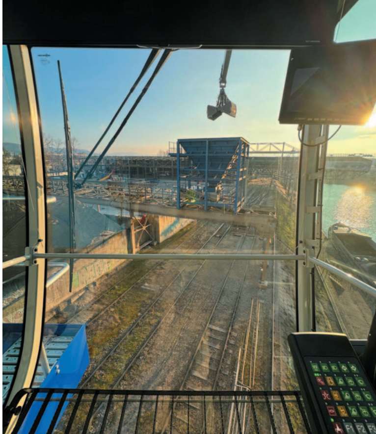
The continuous front and floor windows of the new Portcab cab ensure an excellent view of the working environment.
