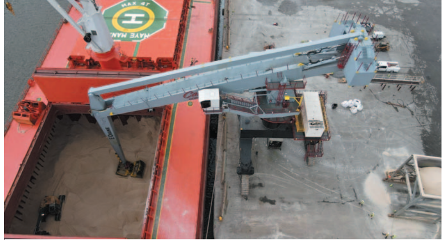
Reaching for the bottom of this Handymax ship is easy and reaching underneath(!) the hatch coamings guarantee full coverage of the bottom of the ship's hold.
