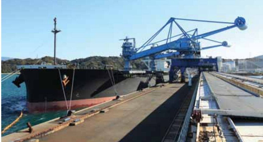
A 3,200tph CSU for Sumitomo, handling coal at a Japanese power station.
