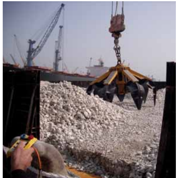
Above: DHM 12m 3 with radio control device. Left, EHS-B 12m 3 electro-hydraulic grab on board. Below, EHS-B 12m 3 grabs on the way to the ship for installation.
