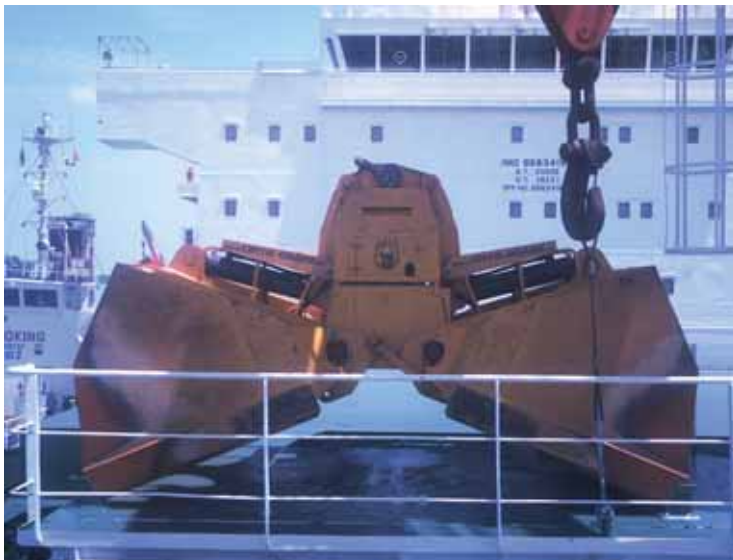
Above: DHM 12m 3 with radio control device. Left, EHS-B 12m 3 electro-hydraulic grab on board. Below, EHS-B 12m 3 grabs on the way to the ship for installation.
