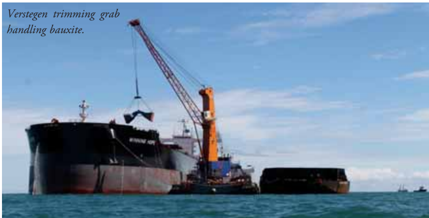
Verstegen trimming grab on a Gottwald floating crane handling bauxite.
