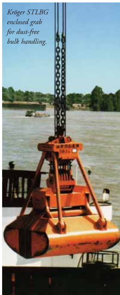
The Kröger STLB four rope grab is ideally suited for bulk handling.
