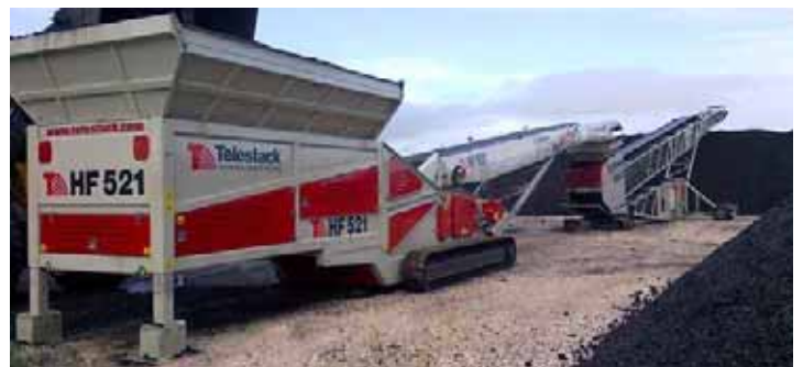
Hopper Feeder & Radial Telescopic reclaiming/ stockpiling coal in stockyard of powerplant
