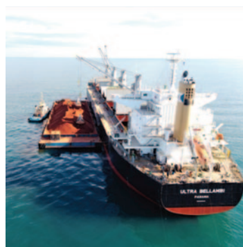
Figure 1: Transshipment example – Dumb Barge & Self-Loading Geared Vessel (courtesy of TSA).
