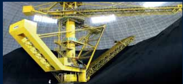
Circular Stockyard with Cantilever Reclaimer
