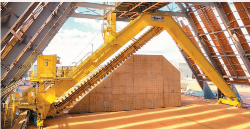
TAKRAF Portal Scraper Reclaimer for the buffer stockyard at a copper operation in the DRC.
