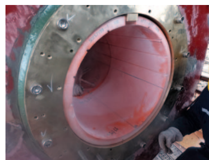
COMPAC Open Seawater-Lubricated Propeller Shaft Bearing System (above).
