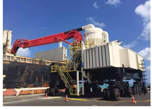
that are installed depends on the maximum allowable wheel loads on the unloading area. Hydraulically operated jacks are installed if necessary to ensure sufficient stability during the unloading process.
