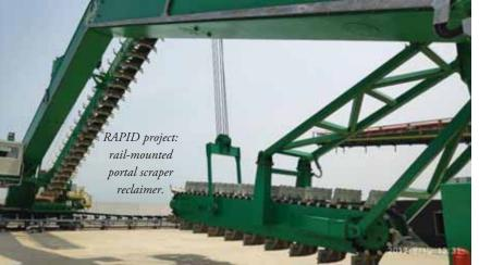
stacking and reclaiming operations. An efficient stockyard must have sufficient amounts of product available with a suitable volume distribution across the stockpiles in order to avoid compromising the reclaiming operation.
