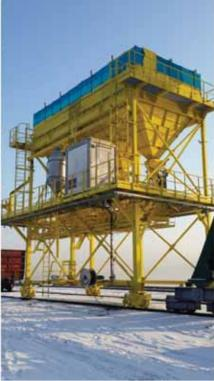
process is handled by the mobile hopper and three 25m-long link conveyors. Emission of dust must be brought to zero, therefore all units are encapsulated and equipped with aspiration, the hopper is equipped with 'flex-flap' grid.
