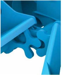
Nemag Clamshell synchronizing system up close. The big advantage of the Nemag design concept – the synchronizing system – has remained unchanged. It is at the heart of the company's clamshell grab's superior performance, guaranteeing 100% symmetrical closure, reduced stress levels in the grab construction and improved digging performance by the grab.
