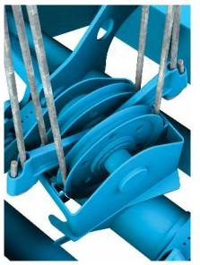
Completely open sheave box of a clamshell grab. The lower sheave box and girder feature a very open and rounded design that greatly decreases the risk of material blocking the pulleys and reduces spillage from the grab whilst travelling to and from the receiving hopper. The benefit: enhanced environmental efficiency.
