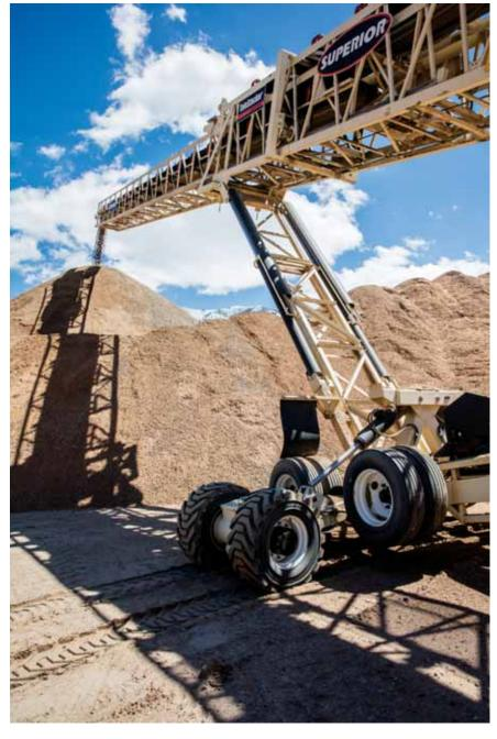
for recycling," says Clayson. He explains that previous to the use of the new TeleStacker Conveyor, they had used a standard radial stacker to stockpile the recycled asphalt, and then they would try to blend the material with the use of a dozer — and even with additional material handling, there was too much discrepancy in the specs.
