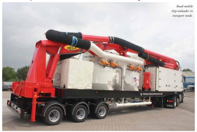
Van Aalst Bulk Handling specializes in the design and supply of equipment for dust-free pneumatic bulk handling of dusty abrasive products. Materials that are handled are cement, fly ash, alumina, china clay, limestone, granulated slag and borax.
