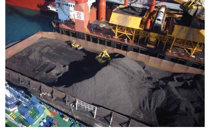
has already verified with manufacturers and classification societies. Furthermore, the cranes can even be replaced by long-arm excavators to take the cargo from barges. Even though their performance is much lower compared to cranes, excavators can be easily procured also on the second hand market and installation on board is extremely easy.
