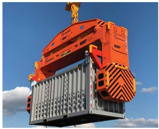
Australian company Container Rotation Systems (CRS) is renowned for its container-emptying system, which offers an efficient solution to the problem of unloading bulk from containers.
