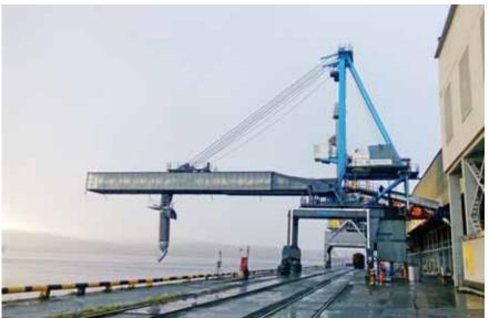
feeding of grain to the conveyor, as well as the variable angle of inclination of the discharging device which provides the equal tight loading of grain inside the ship's hold.
