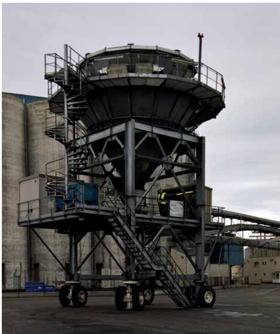
Mobile hopper, travelling on Borghi Assali bogies.
