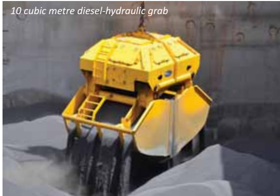
10 cubic metre diesel-hydraulic grab
