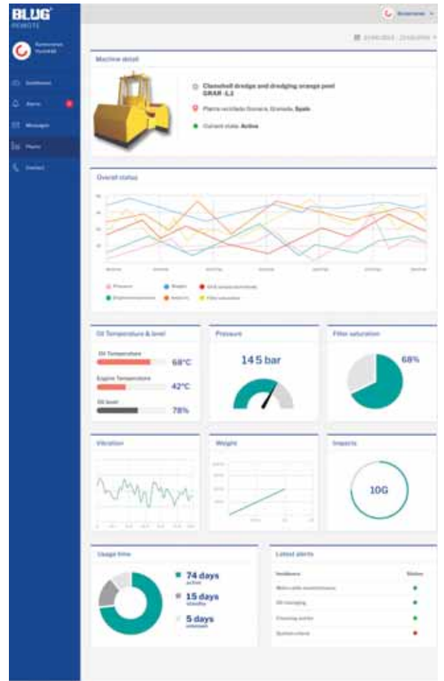
Credeblug's GIITS (Grab Intelligent Interface and Transmission System) connects the grab with the crane control.
