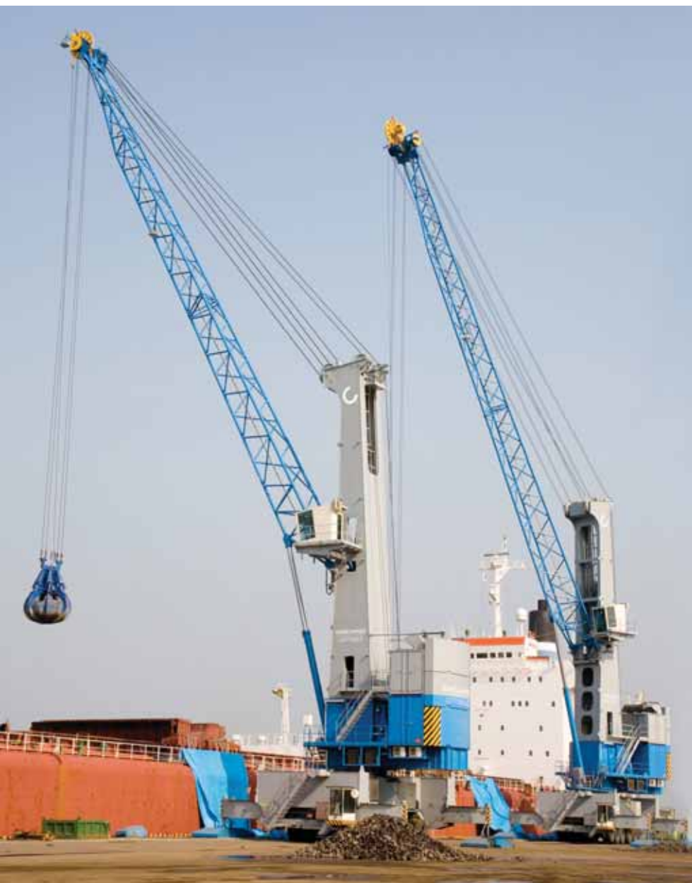
Konecranes Gottwald Model 4 mobile harbour cranes handling bulk material. A similar crane will handle coal and coconut husk in the Japanese Port of Miike.
