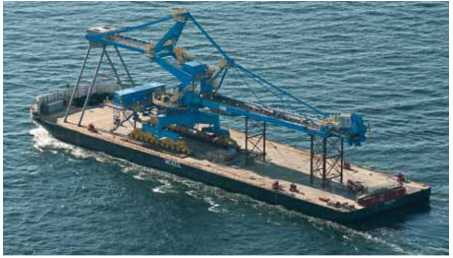
EMS-Tech Inc. delivered a wholly assembled stacker-reclaimer, weighing 1,200 tonnes, to ArcelorMittal Mines via barge in 2013.
