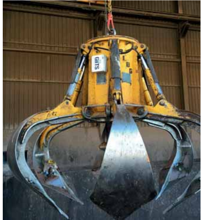
GIITS technology establishes communication via radio-frequency between the handling unit (orange peel grab/clamshell grab/tongs) and the crane, enabling users to have real-time control of different operating modules
