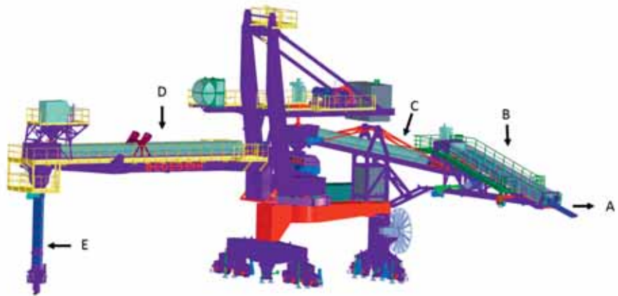
A. Longitudinal belt conveyor installed on the dock; B. tripper lifting the longitudinal belt conveyor installed on the dock; C. Connection belt conveyor between the tripper and the conveyor installed on the shiploader boom; D. Shiploader boom conveyor; E. Loading chute to distribute the material in the cargo hold, that could be telescopic, trimming, slewing and/or tilting.
