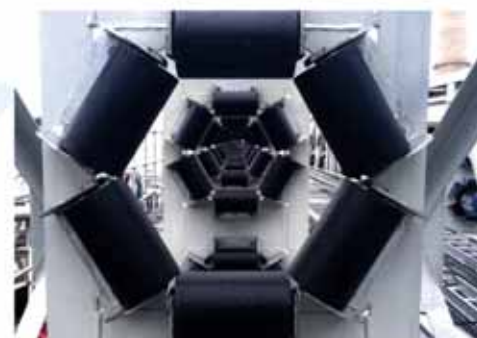
Pipe Belt Conveyor
