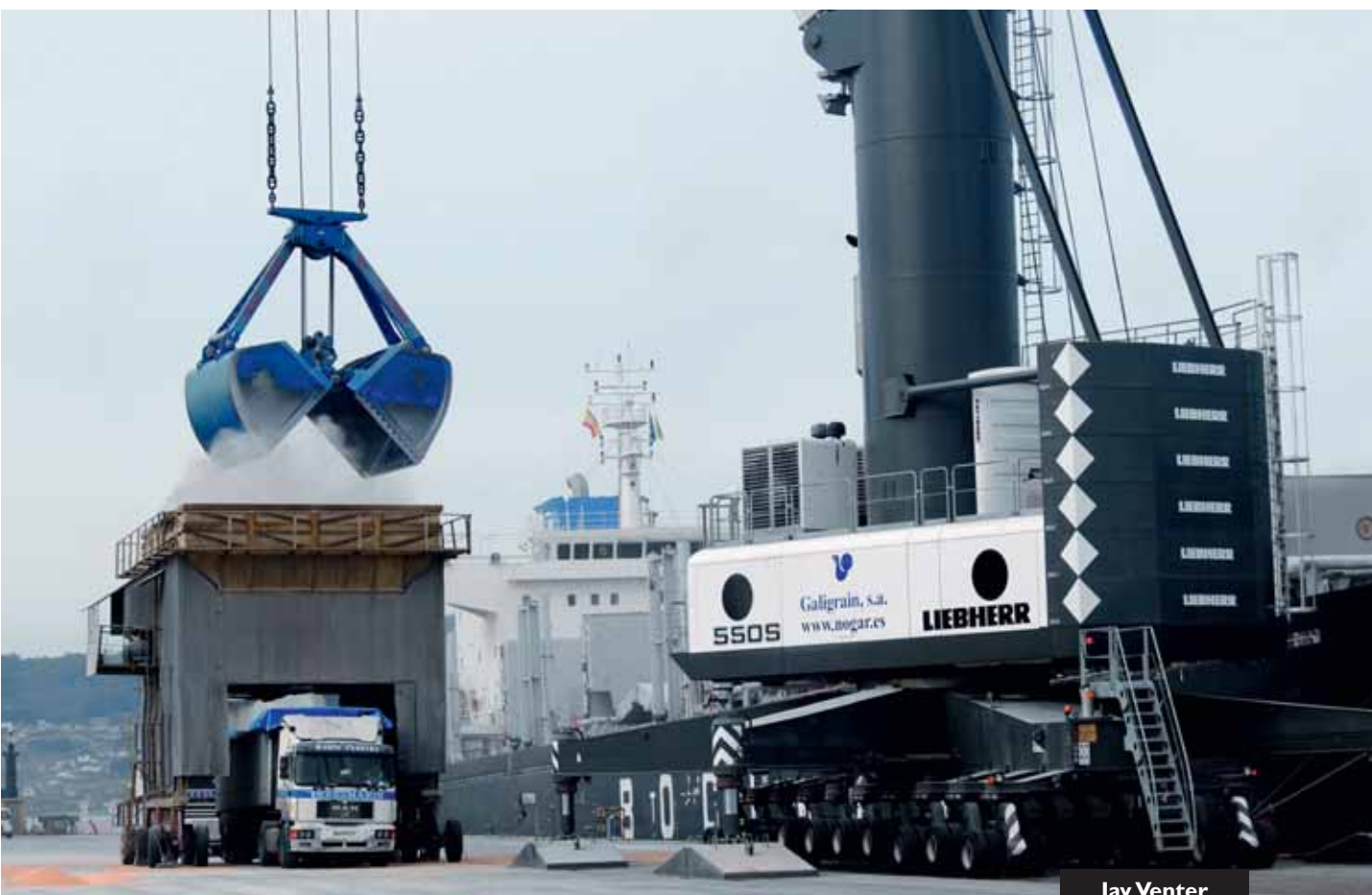
A Verstegen clamshell grab on a Liebherr mobile harbour crane.
