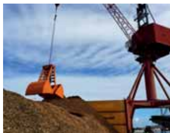
Radio controlled single rope grab: Negrini's radio controlled single rope grabs are ideal for handling all loose materials. They do not require any external power supply, are universal and applicable on all cranes. The radio control manages the opening of the clamshell.
