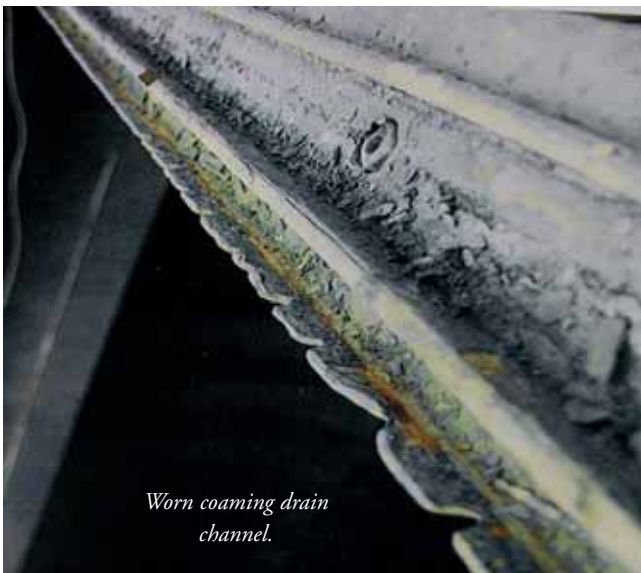
Drain channel, blocked non return drain outlet.
