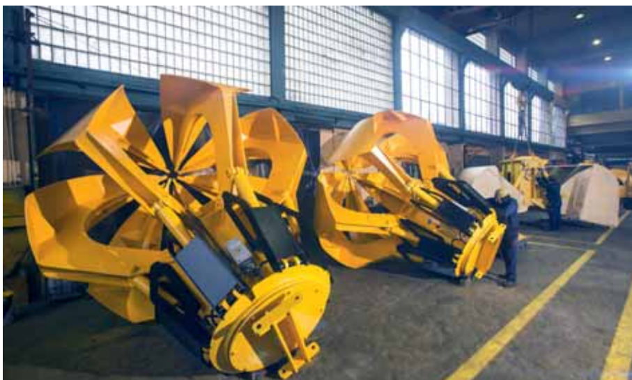
Credeblug recently provided four 10m 3 electro-hydraulic orange peel grabs for the European steel industry.
