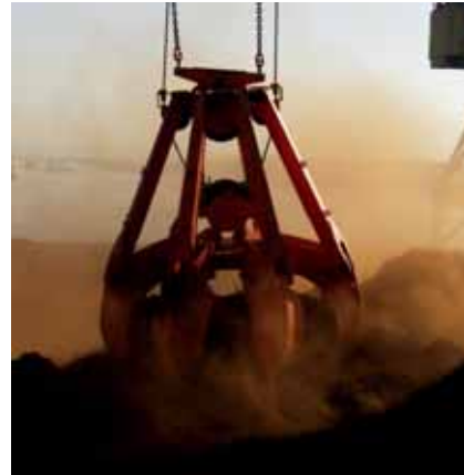
Two- or four-rope orange peel grab: Clamshell grabs can be used for any bulk material, that can be used on all hoisting devices two- or four-rope or crawler cranes.
