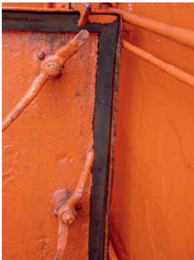
Hatch vent – closed & apparently in good order.
