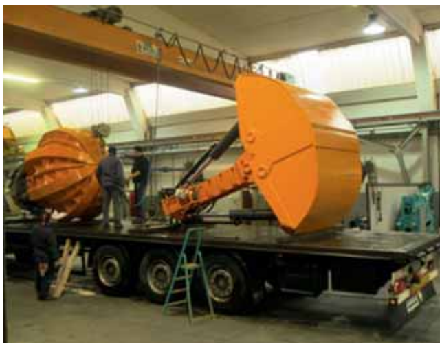
Negrini manufactured an hydraulic clamshell grab and a hydraulic orange-peel grab for the BAUER Group Company in Germany this month.
