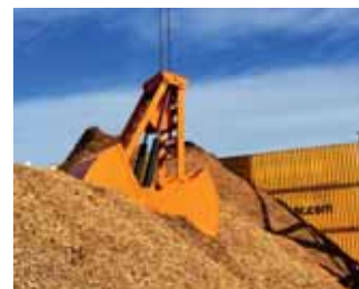
Radio controlled single rope grab: Negrini's radio controlled single rope grabs are ideal for handling all loose materials. They do not require any external power supply, are universal and applicable on all cranes. The radio control manages the opening of the clamshell.
