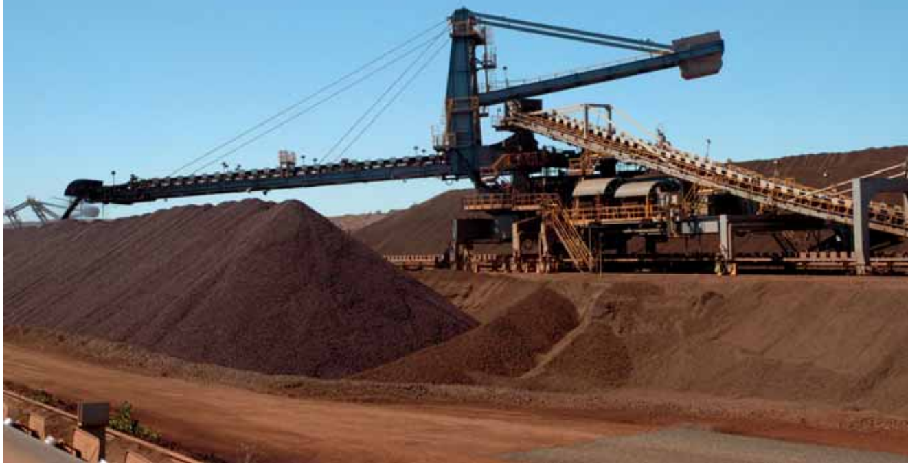
Complete Sandvik stockyard system for an coal export terminal in Colombia.
