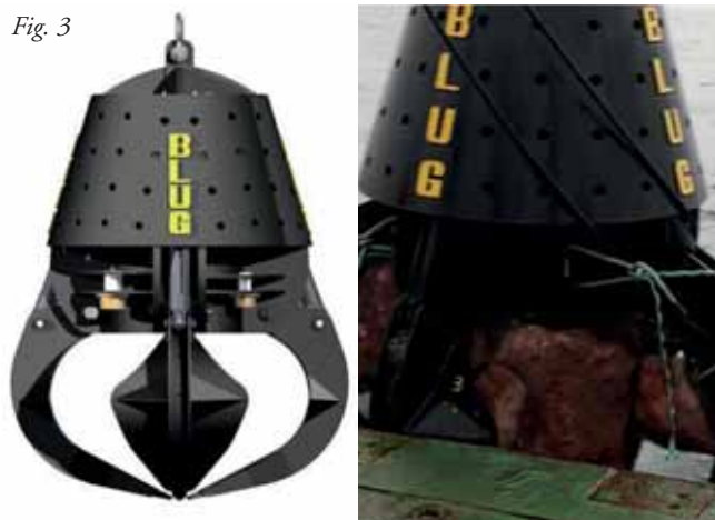
Half-closed design: big volume parts handling, better penetration, smaller contact surface.
