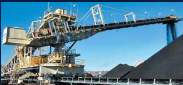
Coal Stacker, Hammer-head Design
