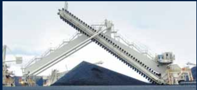
Portal Scraper Reclaimer with Twin-Boom
