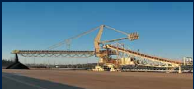
Coal Stockyard with Pylon-type Stacker
