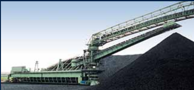
Circular Stockyard with Bridge-type Reclaimer
