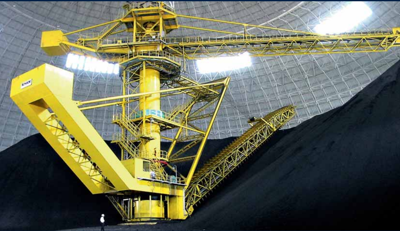
Circular Stockyard with Cantilever Reclaimer
