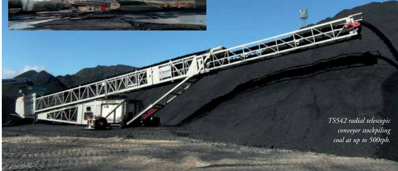
TS542 radial telescopic & HF 521 tracked mobile hopper feeder reclaiming from stockpiles.
