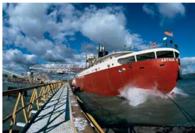
Like many lakers built in the 1950s, the Arthur M. Anderson has been lengthened by nearly 140 feet and converted to a self-unloader (photo courtesy Gary Clark).
