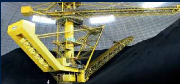
Circular Stockyard with Cantilever Reclaimer
