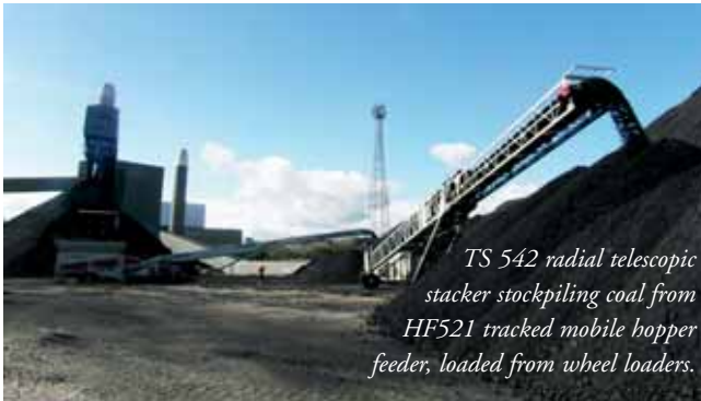
HF 521 tracked mobile hopper feeder feeding TS542 radial telescopic stacker stockpiling at up to 500tph.
