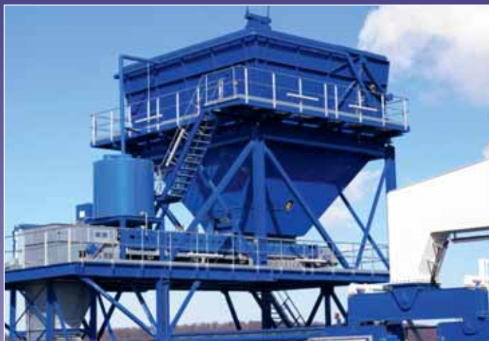
Hopper cars for ship unloading
