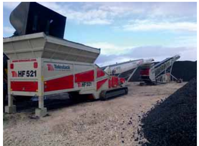
HF 521 tracked mobile hopper feeder feeding TS542 radial telescopic stacker stockpiling at up to 500tph.
